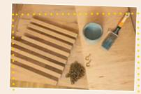
First saw the boards into uniformly sized pieces: Four of the pieces should be as long as the short side of the board. The other four pieces can be a little bit longer.
